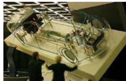
FCVs can be fueled with pure hydrogen gas stored onboard in high-pressure tanks. They also can be fueled with hydrogen-rich fuels; such as methanol, natural gas, or even gasoline; but these fuels must first be converted into hydrogen gas by an onboard device called a "reformer."
