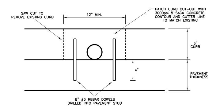
NOTE: THIS CURB DRAIN DETAIL IS TO BE USED FOR STORM WATER RUNOFF ONLY. IT IS NOT TO BE USED AS AN OUTFALL FOR SUBSURFACE WATER OR "FRENCH DRAIN".
